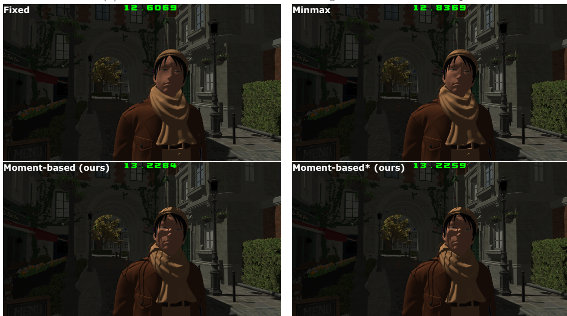
(b) Rendered with four cascades holding 1024 \times 1024 shadow maps
